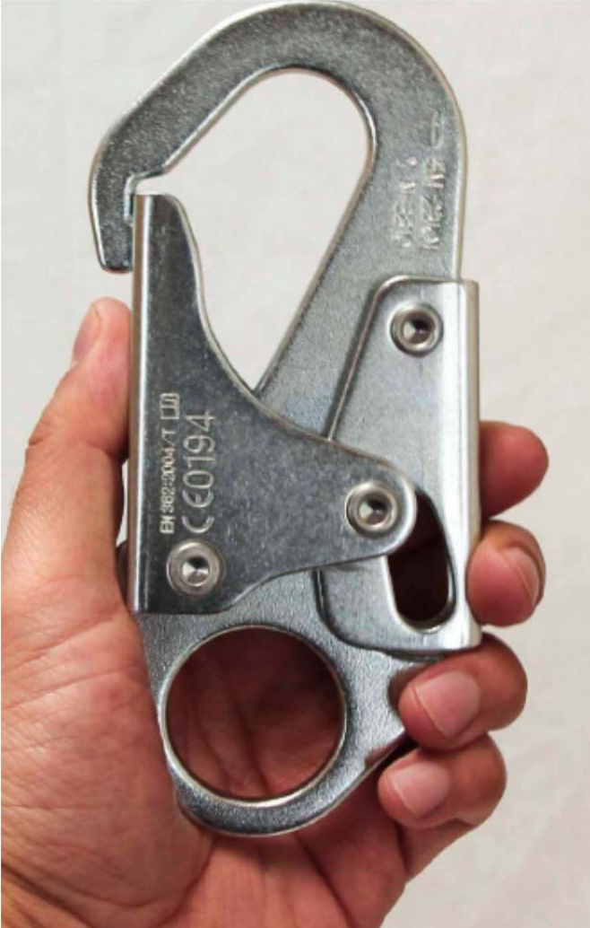
Figure 5: Picture of hook with “tail” of rivets exposed
