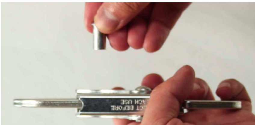
Figure 7: Fully removed rivet
