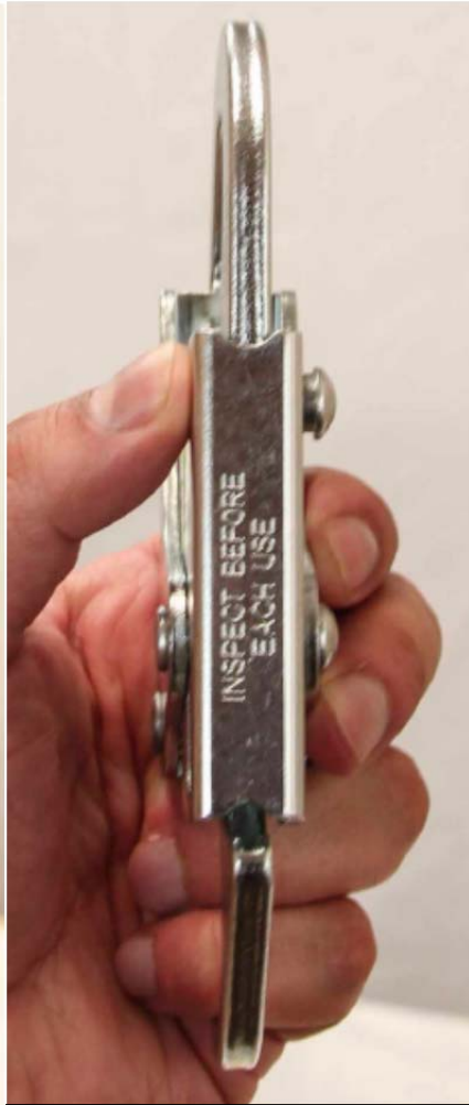
Figure 6A: Attempt with pressure to unseat rivet
