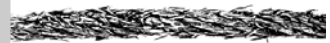
Too long in service. Repeated winding and unwinding of this rope on a drum while it was under heavy stress caused the unusually severe wear shown.
