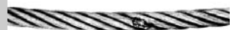
Poor work procedures. Damage to strands and wires resulted from electric arcing.
