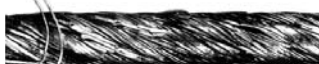
Infrequent inspection. Neglect of periodical inspection left this rope in service too long, resulting in considerable abrasion.
