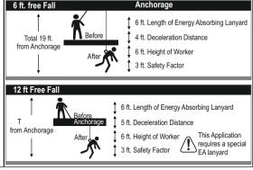
Swing Falls: Swing fall occurs when the position of the anchorage point is not directly above the point where a fall occurs. In such
