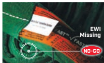
EWI IS MISSING: REMOVE FROM SERVICE
