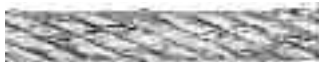
Lack of lubrication. Premature breakage of wires resulted from "locking" of strands, which was caused by insufficient lubrication.
