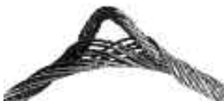
Too sudden load release. The sudden release of a load cause birdcaging. Here individual strands open away from each other, displacing the core.
