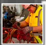
Our trained and experienced rigging and fall protection experts offer inspection services for all of your wire rope, chain, synthetic slings, rigging hardware and fall protection gear. Our inspection teams provide written records of our inspections in according with ASME B30.9 (Slings), B30.16 (Overhead Hoists), B30.21 (Manual Lever Operated Hoists), and B30.26 (Hardware), OSHA 1926, OSHA 1910 and Manufacturers' Recommendations.
