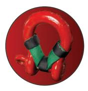
The pin area of a shackle can damage synthetic slings. Placing synthetic slings on the pin should be avoided. Shackles may have a sharp edge where the pin goes through the shackle ear. If the sling is rigged on this area, it could become severely damaged. If you must rig on the pin, protect your sling with a **Shackle Pin Pad**.
