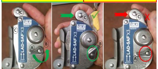
Proper operation of the sleeve is shown in green above. The locking lever (A) must be rotated to position (B) for the side plate (C) to be pulled backwards. If your sleeve functions in this manner, it is working properly. If you are able to pull the side plate (C) back by pulling on the top roller without first rotating lever (A) to position (B), then the unit should be removed from service (see red example above).
