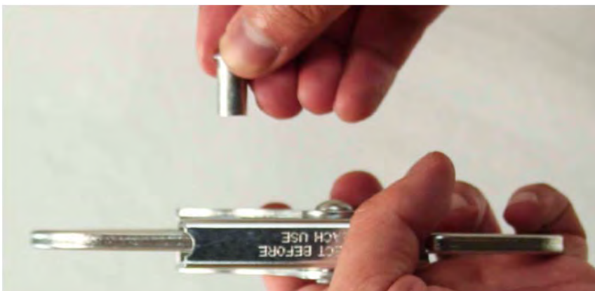
Figure 7: Fully removed rivet
