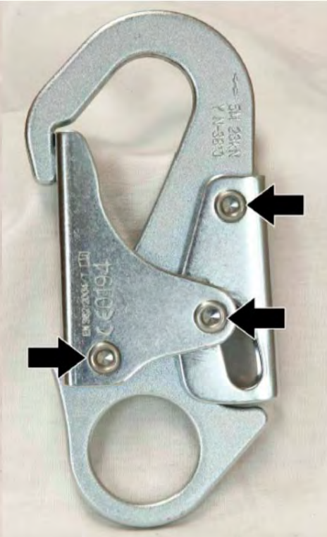
Figure 4: typical pressed "tail" end rivet locations on stamped hook
