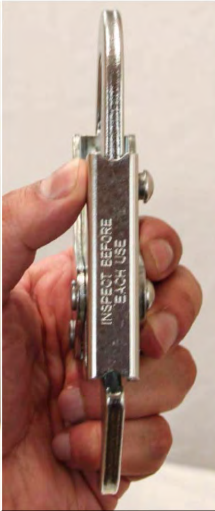
Figure 6A: Attempt with pressure to unseat rivet
