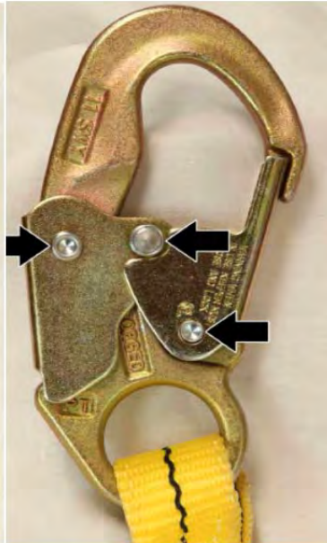
Figure 4A: typical pressed "tail" end rivet locations on forged hook
