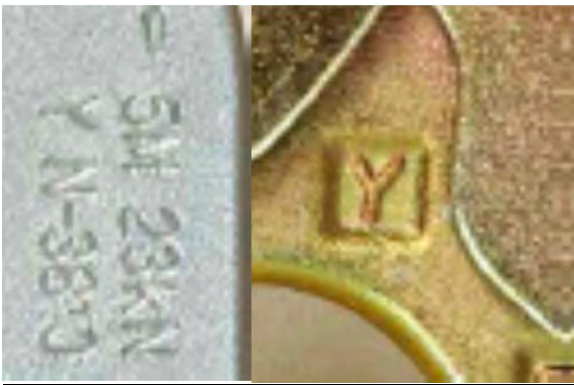
Figure 2: Typical YOKE Industrial Corp. hook markings.
