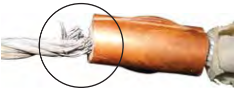
Cable fraying at swage contact point
