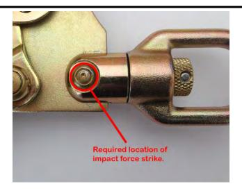
In our investigation, a hook with damaged nut by impact force will exhibit symptom of abnormal gap/tolerance on the bolt / nut assembly. We kindly ask you to incorporate the below additional inspection procedure to your current ones.
