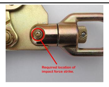
In our investigation, a hook with damaged nut by impact force will exhibit symptom of abnormal gap/tolerance on the bolt / nut assembly. We kindly ask you to incorporate the below additional inspection procedure to your current ones.
