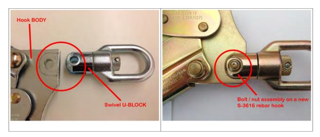
Our production process requires the end of the threaded bolt to be spun down by an orbital press to guard against removal of the nut. In addition, locitite is applied to the bolt thread. Dis-assembly requires deliberately grinding off a part of nut and hammering out the bolt by force.
