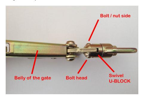
3. Press your thumb against the bolt head and push it upward. If there is abnormal gap/tolerance, you should feel it immediately where the bolt could be move up and down loosely in the Swivel U-BLOCK. Continue pressing your thumb against the bolt head and visually inspect the bolt / nut side. Please reference photos in step 4 for damaged units and step 5 for good units.
