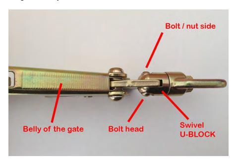
3. Press your thumb against the bolt head and push it upward. If there is abnormal gap/tolerance, you should feel it immediately where the bolt could be move up and down loosely in the Swivel U-BLOCK. Continue pressing your thumb against the bolt head and visually inspect the bolt / nut side. Please reference photos in step 4 for damaged units and step 5 for good units.
