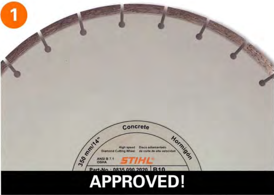
Photos #1 and #2 show examples of recommended STIHL diamond abrasive wheels that grind material. Note that the cooling slots and segments on such diamond wheels are NOT cutting teeth.
